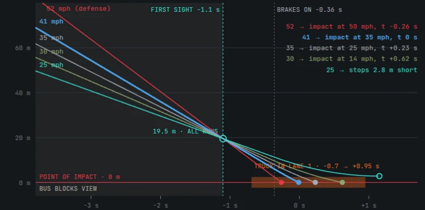
TIME-DISTANCE • SEDAN NOSE TO POINT OF IMPACT • TRUCK IN LANE 1 SHADED
